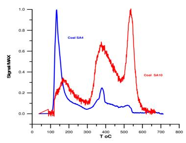
Thermospectra of mercury in bituminous coal from Vaal (SA4, total Hg 540 ppb) and Highveld (SA10, total Hg 195 ppb) coal fields (South Africa).
